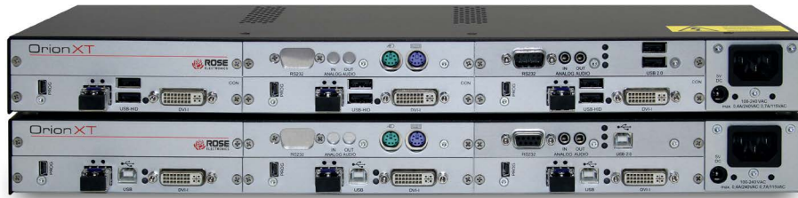
Figure 3. Various cards installed in six card chassis
