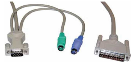
High resolution PC PS/2 cable – Computer to switch
